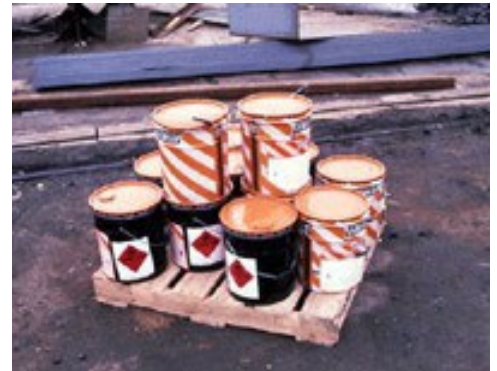
Flammable materials stored in fire-resistant containers.
