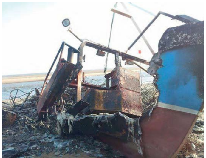
Figure 2: Burnt out wreck of a fishing vessel (looking aft)
